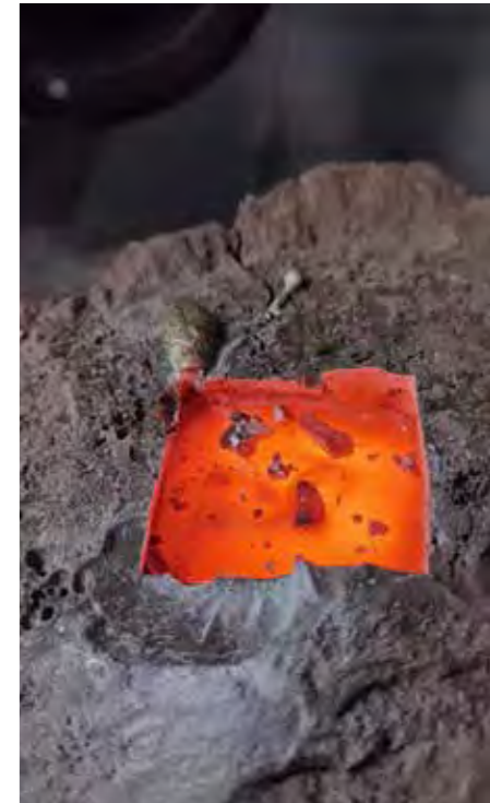
Center left to right: Fraunhofer IWS explores remote contact-free solutions using a laser source to separate contaminated material. In addition to questions regarding the configuration of output power, cutting head, focal length, and cutting angle, the research team is investigating the cutting quality and the melt pool.
