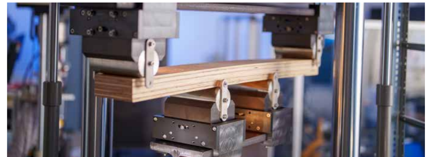
The competence field materials characterization and testing at Fraunhofer IWS investigates the fatigue strength of wood-based materials in load-bearing structures by means of bending tests, for example.
