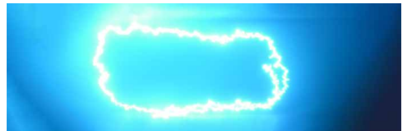
A magnetically controlled arc discharge moves across a rectangular cathode, creating plasma that is used for coating.
