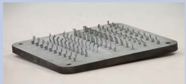
Base plate with Laser Powder Bed Fusion-printed mandibular distractor pads made of TiAl6V4.
