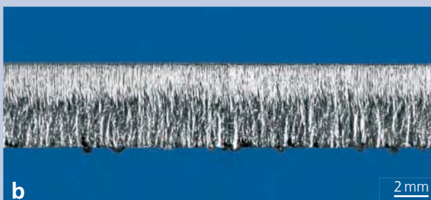
Cutting edge of a 5 mm specimen (a) without burr adhesion and (b) with burr adhesion.
