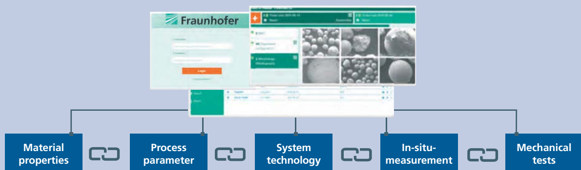
Infrastructure of the process information management system for the individual steps in the additive process chain
