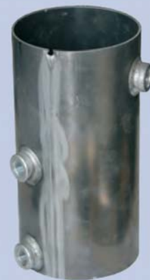
Weld seams of an air reservoir for truck brake systems, which can be analyzed with the AZOM measuring system.
