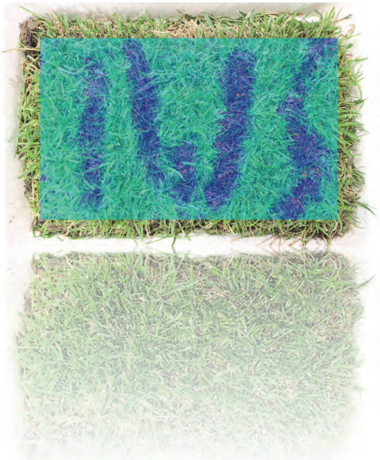
Embedded in grass, the "IWS" writing was made of synthetic turf and visualized by hyperspectral imaging
