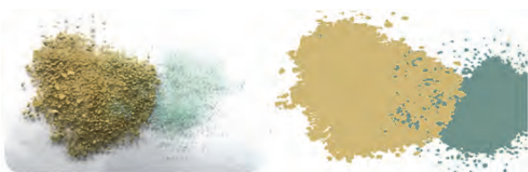
Crystalline powder of metal-organic frameworks, left : visual image, right : classified HSI image
